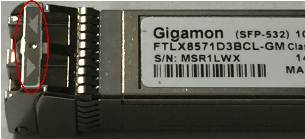
Figure 1: Transceiver With Incoming and Outgoing Arrows
